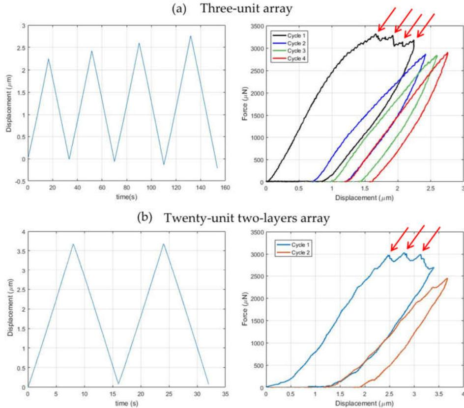
**Figure 9.** Mechanical responses revealing microcrack and fracture. (a) Imposed displacement-time and force-displacement plots for a three-unit array (cf. Video S5: Three-unit cracking). (b) Imposed displacement-time and force-displacement plots for a twenty-unit two-layer array (cf. Video S6: Twenty-unit two-layer cracking). Arrows indicate fracture events during the deformation.
