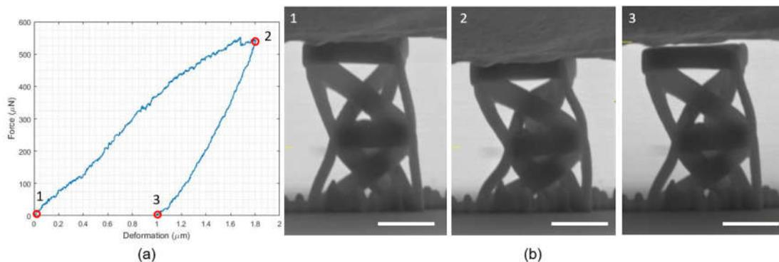
**Figure 6.** Mechanical testing on a single unit cell. (a) The force-displacement plot for an individual unit. (b) Snapshots of the structure at different times during testing (cf. Video S2: Individual unit). The white scale bar for each SEM figure is  $5 \mu\text{m}$ .
