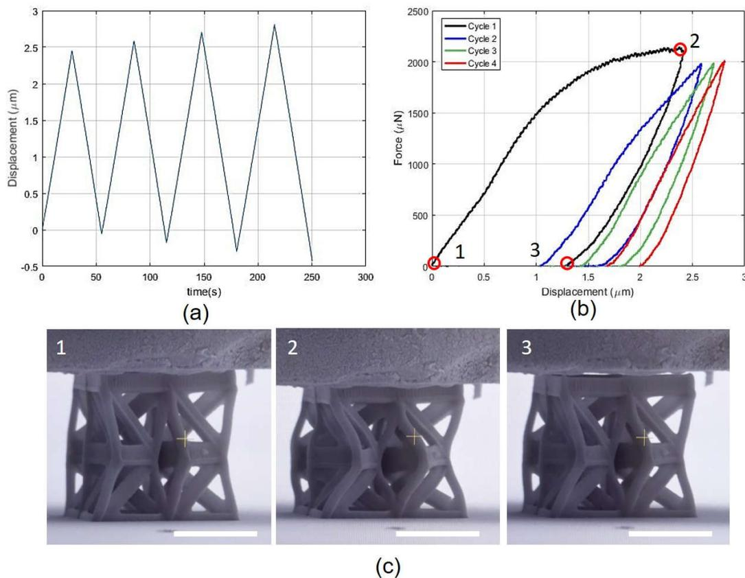
**Figure 7.** Mechanical testing on a three-unit array. (a) Imposed displacement vs. time and (b) force vs. displacement plots. (c) Snapshots of the sample during testing (cf. Video S3: Three-unit array). The white scale bar for each SEM figure is  $8 \mu\text{m}$ .
