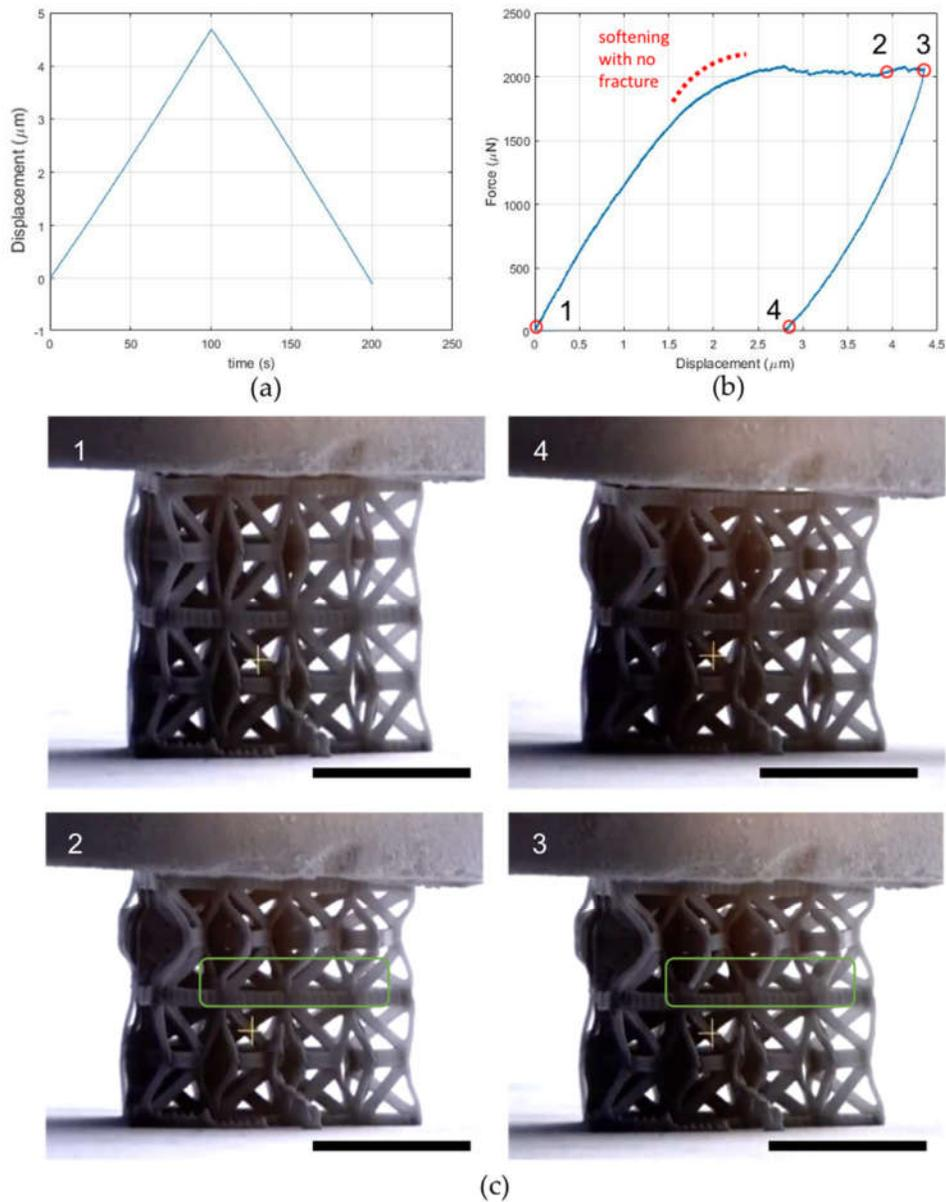
**Figure 8.** Mechanical testing on a twenty-unit two-layer array. (a) Imposed displacement–time and (b) force–displacement plots. (c) Snapshots of the sample during testing (cf. Video S4: Twenty-unit two-layer array). Some fracturing beams are enclosed in the green rectangle. The black scale bar for each SEM figure is 10 μm.
