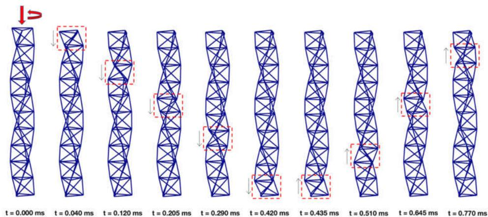
**Figure 11.** Snapshots extracted from the video of the motion of a column of ten bistable prisms impacted with initial vertical and angular speeds at the top base (see also Video S7 of Supplementary Materials).
