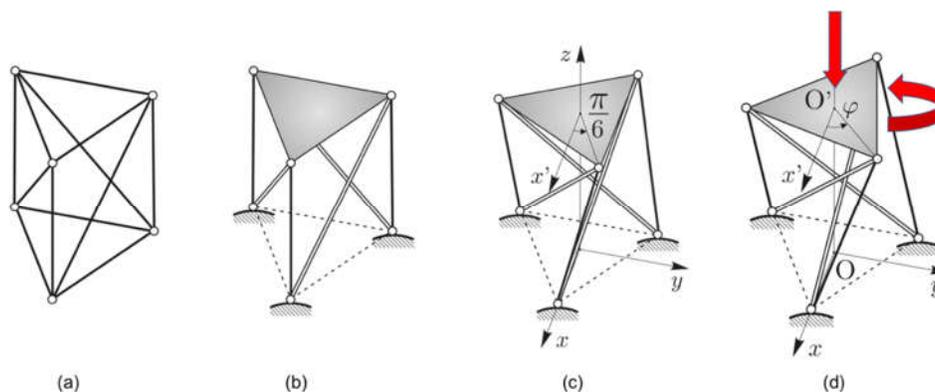
**Figure 2.** Design process of a tensegrity structure. (a) A bar framework in the shape of a regular right prism. (b) A corresponding right-handed tensegrity prism with cables (single line) and bars (double line). (c) Prestress-stable equilibrium configuration of the tensegrity prism. (d) When the internal mechanism is activated, the top triangle rotates about and translates along the vertical three-fold symmetry axis.
