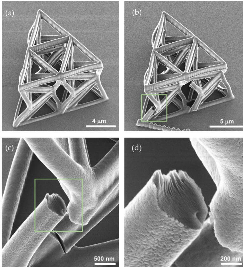
**Figure 10.** Helium ion microscopy (HIM) images of a three-unit array after testing. (a) HIM imaging of a structure that fracture did not commence. (b,c,d) HIM images of a fractured sample.
